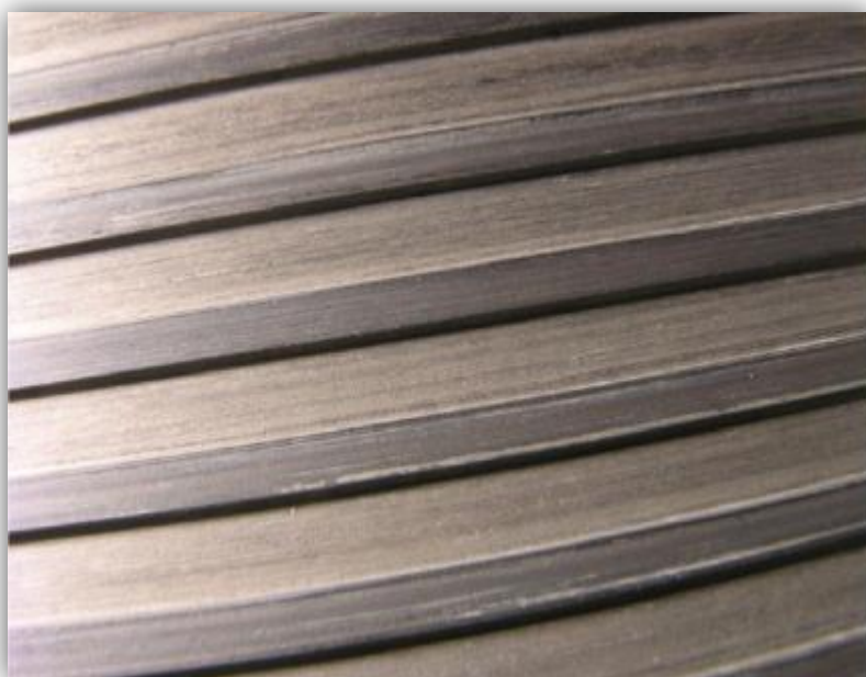
Gun Barrel 066 after Automatic Cleaning System was applied (12 Passes)
